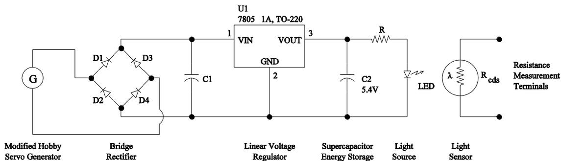
1. In the first step, the generator was characterized. Voltage across the terminals was related to speed and direction of the generator cranking action. Polarity of the voltage depends upon cranking direction, and the magnitude upon the speed. Participants connected a particular LED and current-limiting resistor to see how the cranking speed and direction affect brightness.
