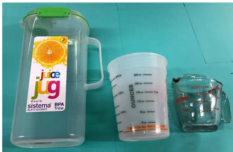
Figure 5 Examples of common household measuring devices used for pump flow measurement.
