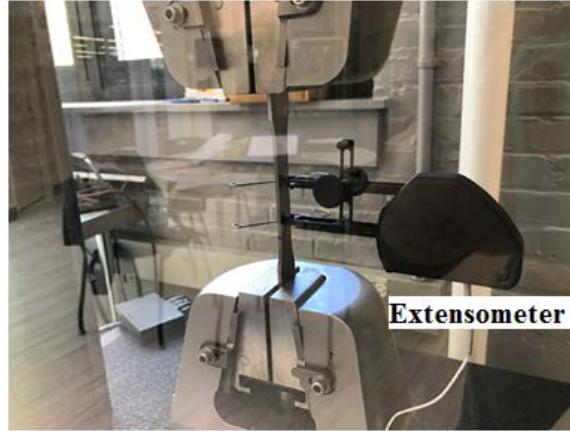
Figure 3: sheet-type tensile test with extensometer
