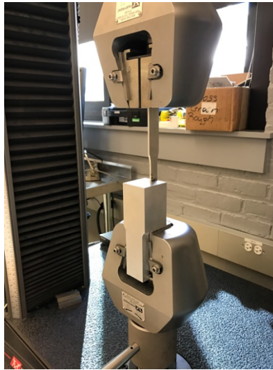
Figure 4: auxiliary block for vertically assembling the specimen
