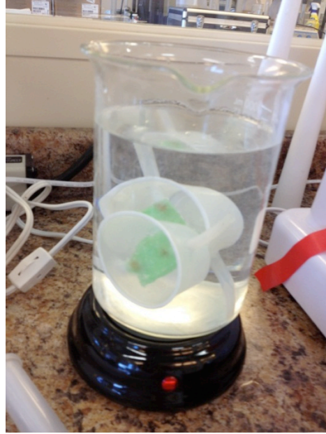
Figure 3: Dissolving the cotton candy in a water bath. We use a beaker sitting on a coffee cup warmer as shown.
