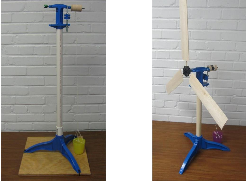
**Figure 1: Example configurations of the windmill assembly used in ENGR 111.**
