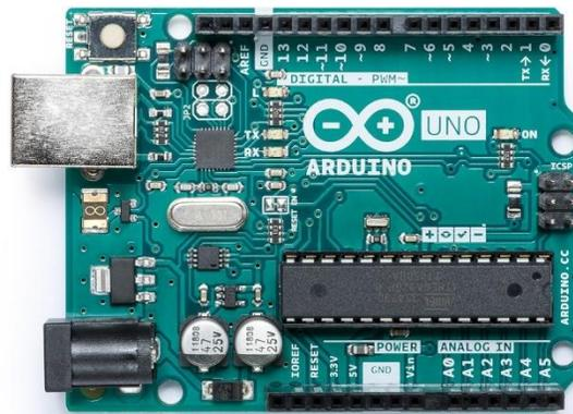
*Figure 1: Arduino Uno Microcontroller*
