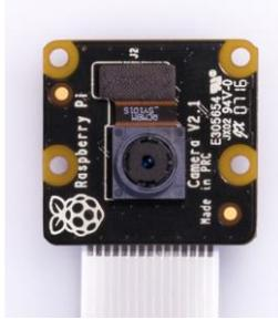
Figure 2 - RaspberryPI NoIR Camera V2
