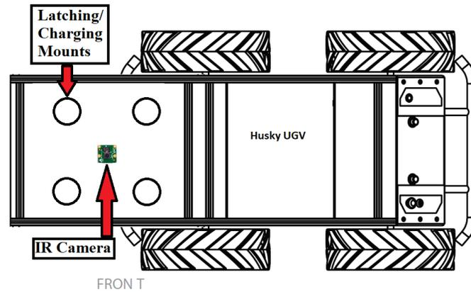
Figure 4 - UGV Functional Diagram
