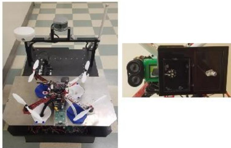
**Figure 3 - Husky with UAV Top View, Bottom View of UAV with Tracking LEDs**
