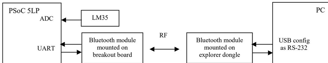
Figure 13 – Block Diagram for Remote Control System
