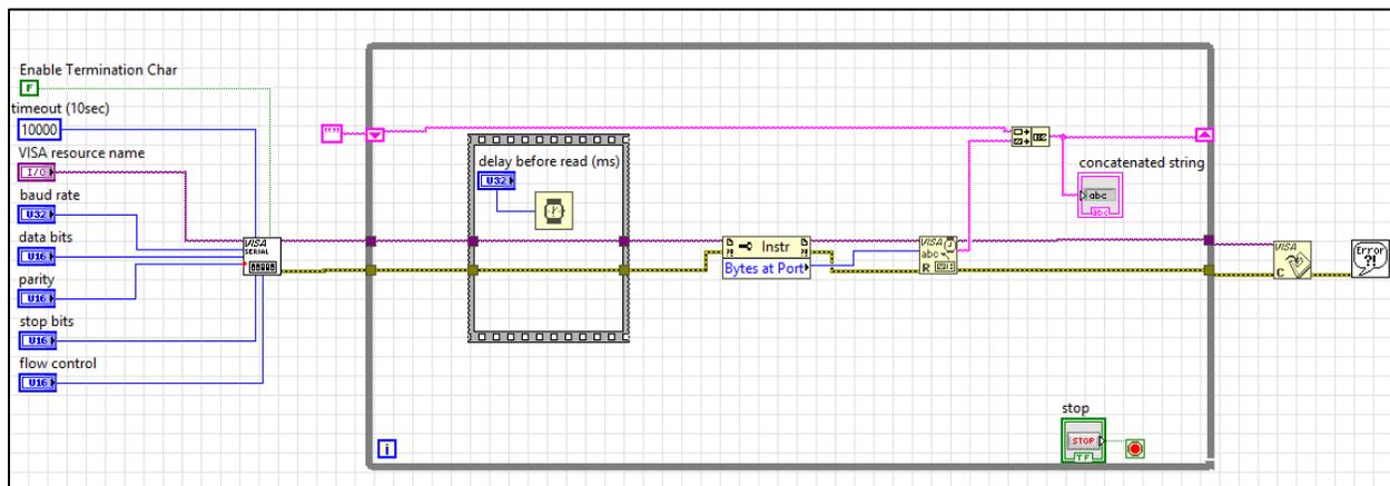
Figure 12 – LabVIEW Program for IR Communications System
