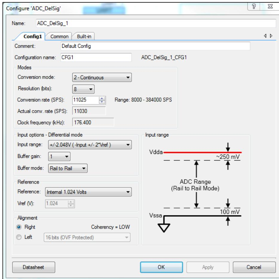
Figure 6 – ADC Configuration for Audio Data Collection
