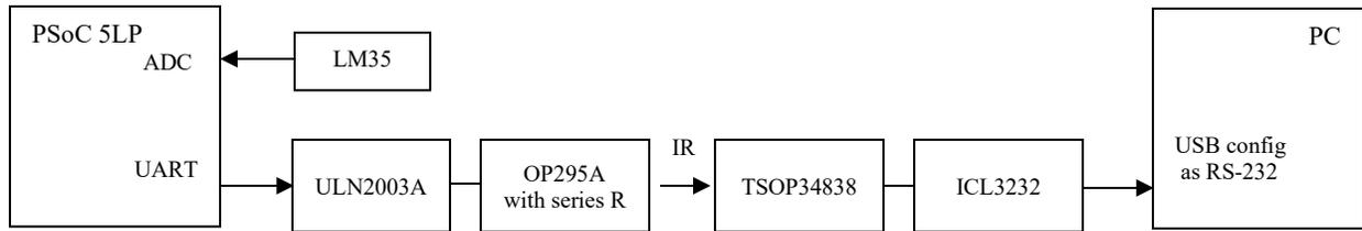
Figure 9 – Block Diagram for IR Communications System
