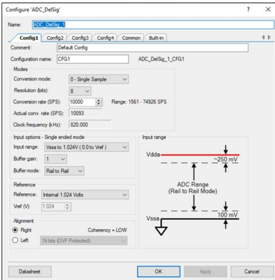
Figure 2 – ADC Configuration for Temperature Data Collection
