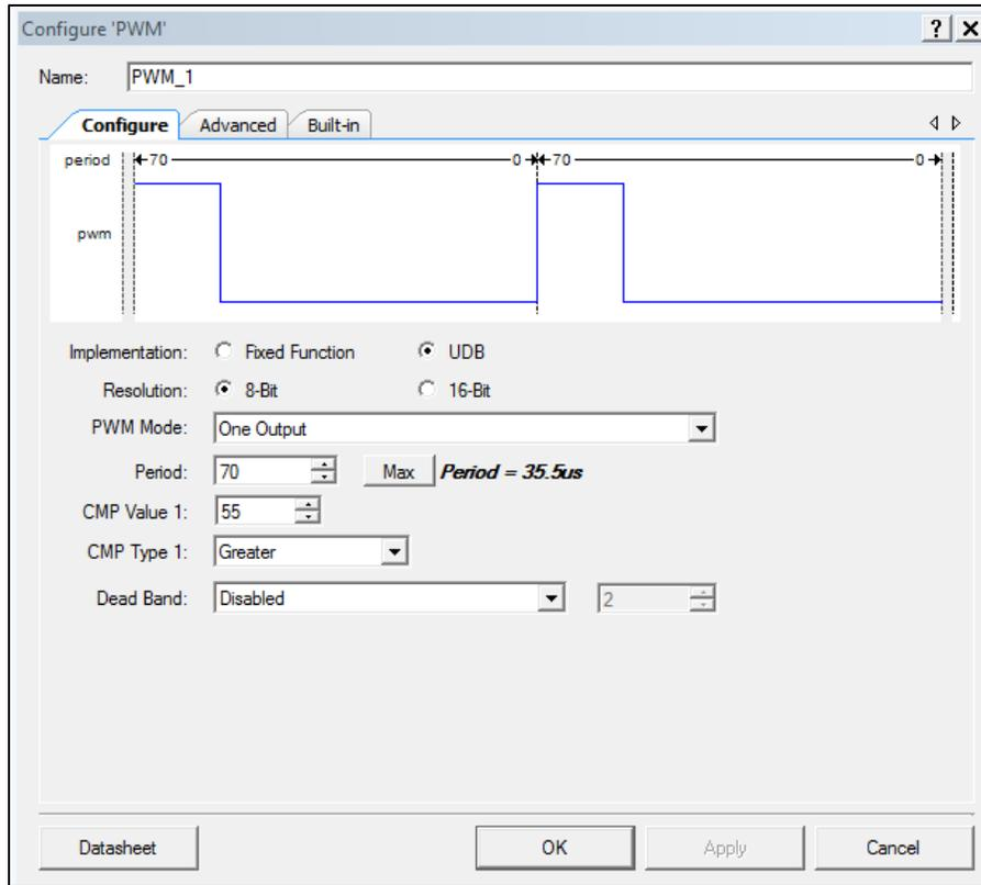
Figure 11 – PWM Configuration for IR Communications System
