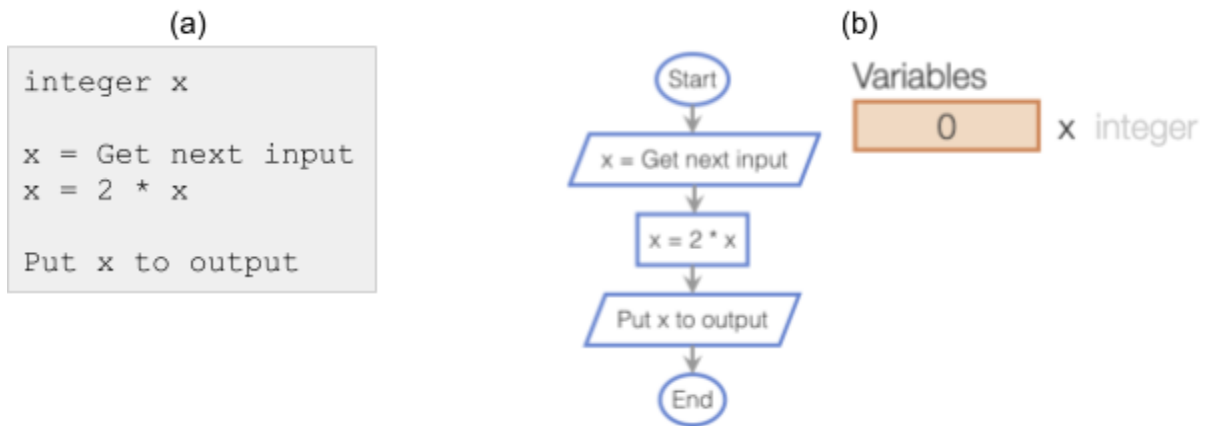
Figure 4: Sample program that prints double the value of the input value in (a) textual code and (b) flowchart.
