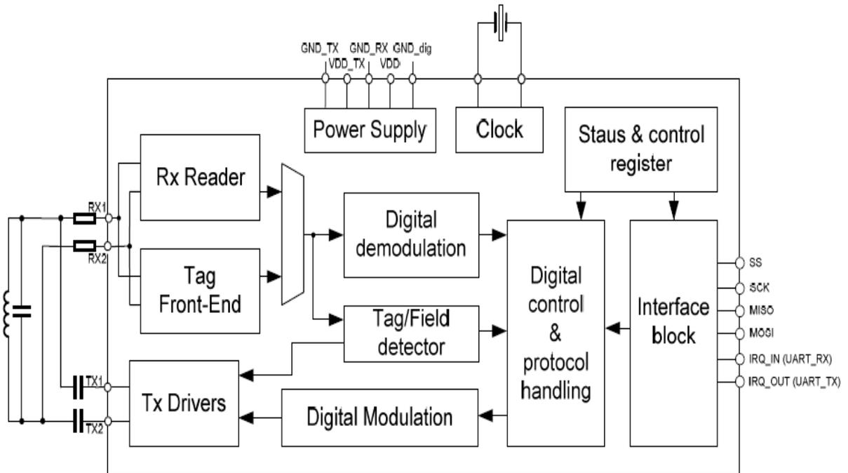
Figure 1: The Melexis RF evaluation board schematic diagram
