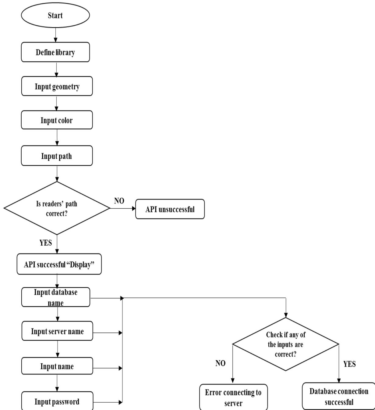
Figure 3: Merging API with the database connection
