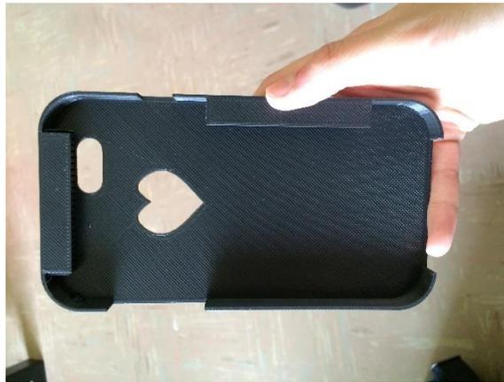
Figure 1: 3D Printed Phone Case from Project #2 of a first-year engineering design course
