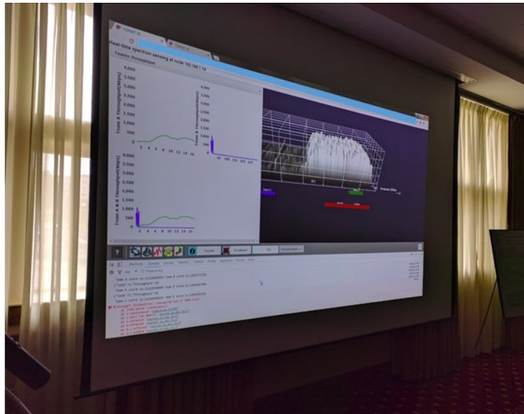
Figure 5. From the final competition in 2017: Large projection screen showing real time performance of participants' radios. Participants and spectators observe instantaneous throughput and cumulative throughput as well as a three-dimensional view of spectrum showing the interferer.
