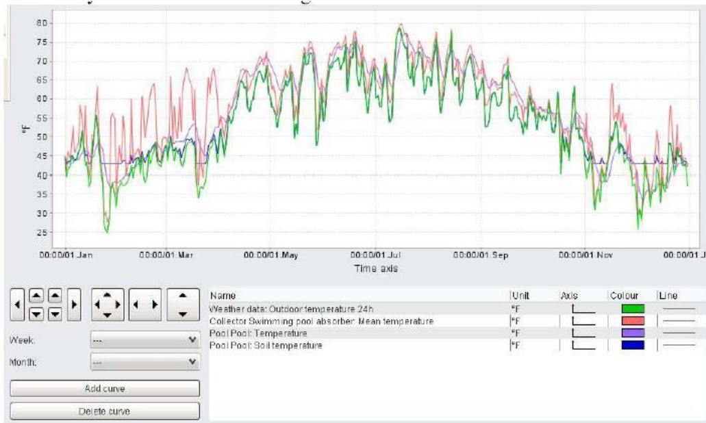
Figure 9 A sample graphical representation of various temperatures of the system
