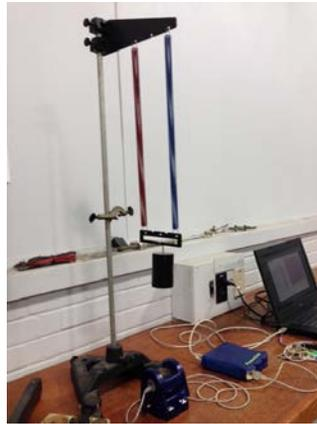
Figure 3 Photograph of the dynamic response of a 2<sup>nd</sup> order system experiment
