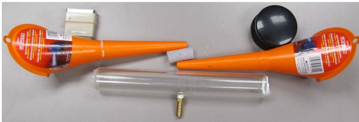
Figure 3. An Exploded View of the Venturi, Including Funnels, Connecting Tube and the
