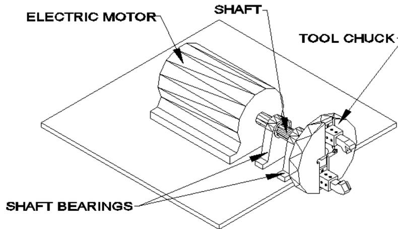
Figure 2: The Rotating Tool Assembly
