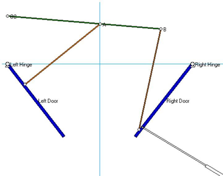
**Figure 9** Barn Door Mechanism Example
