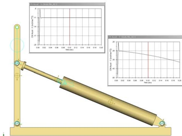
**Figure 11** COSMOS/Motion Model of Cylinder Mechanism
