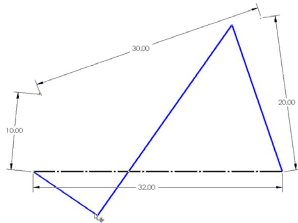
**Figure 3** Finding Range of Motion of Link 2
