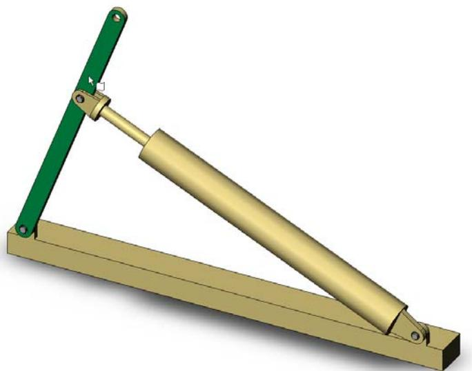
**Figure 6** 3-D CAD Model of Cylinder Mechanism
