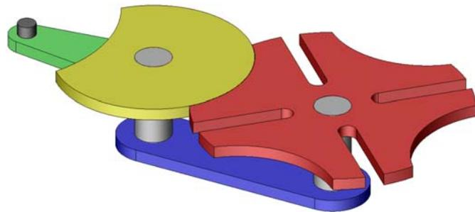
**Figure 8** Geneva Wheel Mechanism Model
