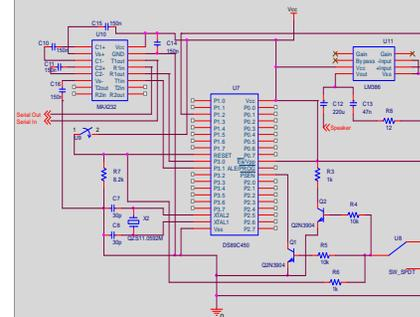
Schematic for Synchronous 8051 Microprocessor and Supporting Circuitry
