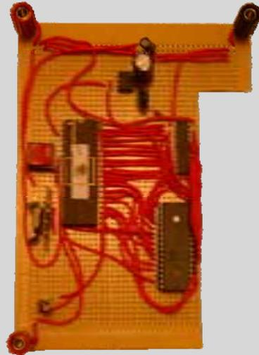
Asynchronous 8031 Microprocessor and Supporting Circuitry on Breadboard
