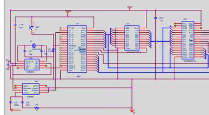
Schematic for Asynchronous 8031 Microprocessor and Supporting Circuitry
