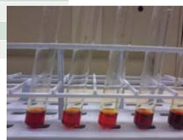
Figure 6. Samples treated with 3,5-dinitrosalicylic acid. Note the differing color changes.
