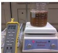
Figure 3. Sample of switchgrass hydrolyzing in a heated acidic solution.
