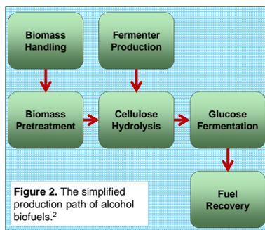
Figure 2. The simplified production path of alcohol biofuels.<sup>2</sup>
