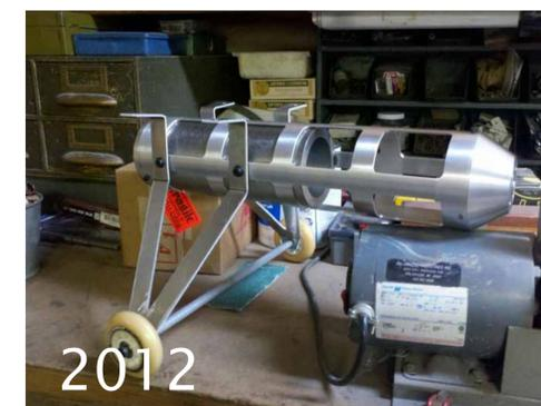
The landing gear design focused on reducing the number of components to reduce weight. By combining the wing mount and landing gear, the number of parts was reduced from thirteen to three. This reduced weight by 45%.
