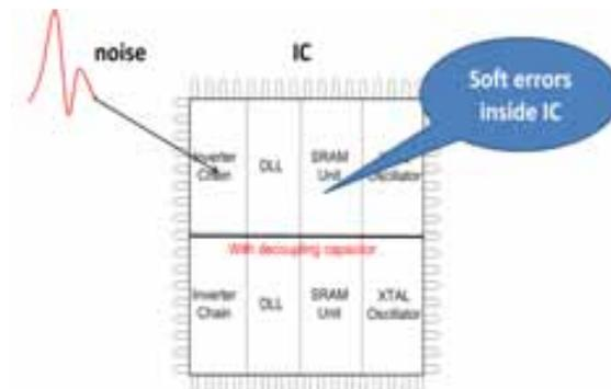
Figure 1. Overall architecture of the test IC.
