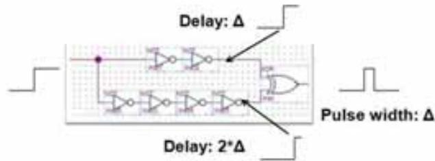
Figure 2. Faster-than-the-clock signals can be built using glitching.
