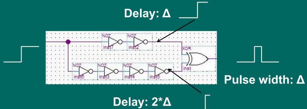
Fig. 4. Signals built using glitching
