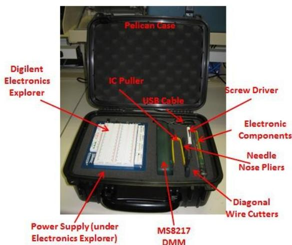
Figure 2: Portable electronics self-contained lab components utilizing the Electronics Explorer™ Board.
