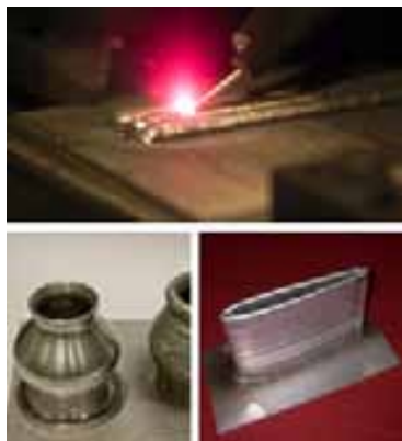
Top: EBF 3 during a deposit Bottom: Parts that have been fabricated using EBF 3 [3]
