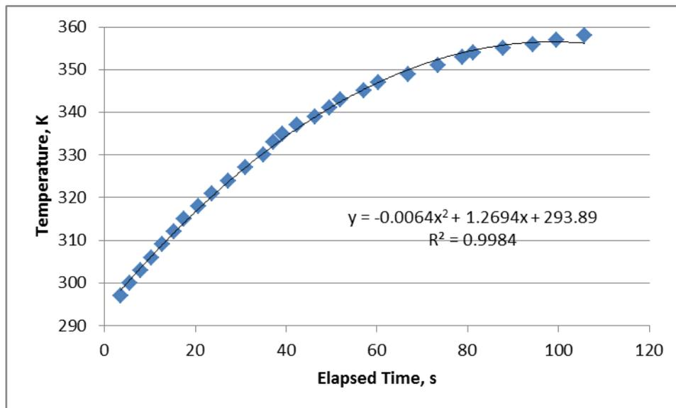
Figure 4. Plot of Experimental Data: Bulb Surface Temperature as a Function of Elapsed Time
