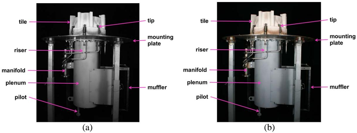
Figure 5. Photographs of a process burner: (a) black-and-white and (b) color.
