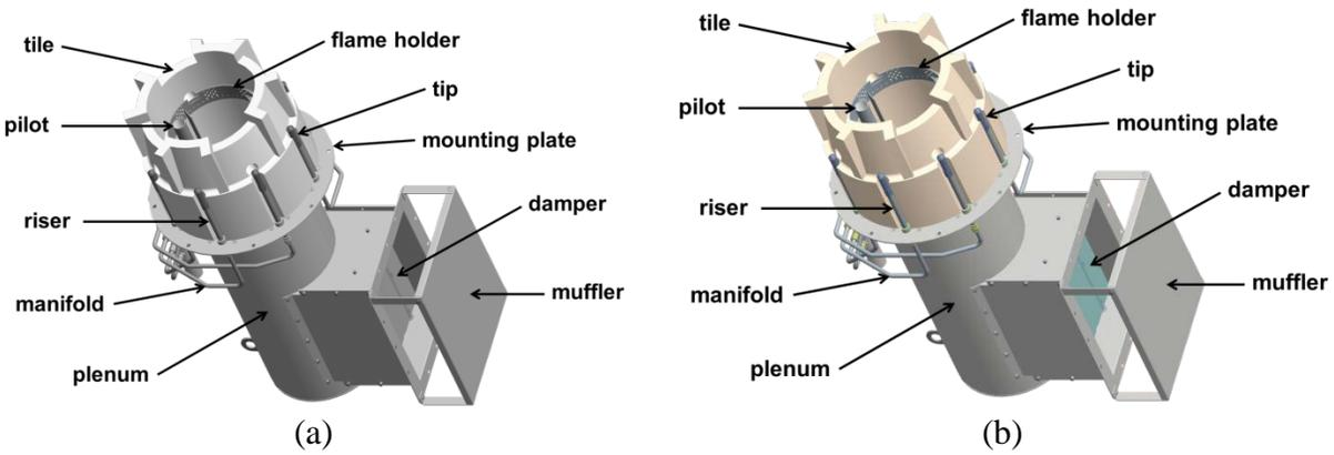
Figure 7. 3D drawings of a process burner: (a) black-and-white and (b) color.
