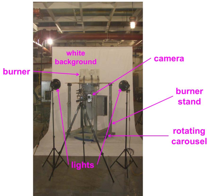
Figure 3. Setup for taking burner photos to make an object movie.
