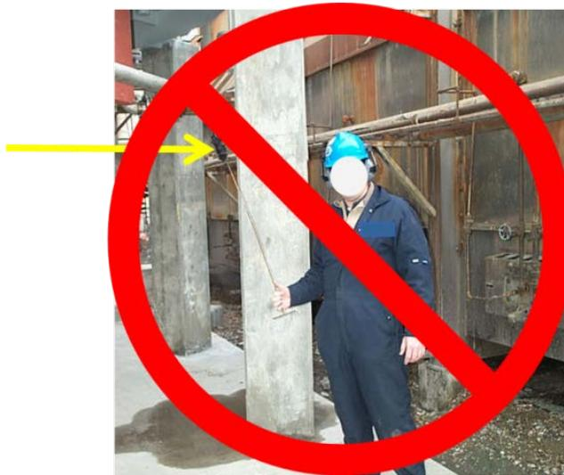
Figure 10. Photograph of an operator holding a rag on a stick, which is improperly used to light a process burner.
