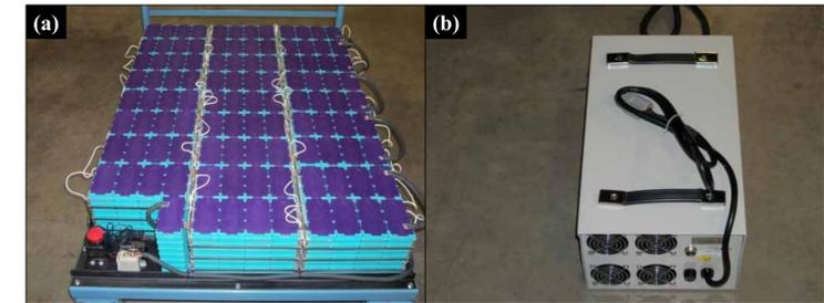
Figure 8: Photograph (a) shows the LiFeMnPO4 battery pack used in the second generation EV and (b) custom 105 cell battery charger on the right. The batteries can be recharged using a standard 120/240 V electrical outlet. This battery bank will eventually be placed in the trunk of the second generation EV.
