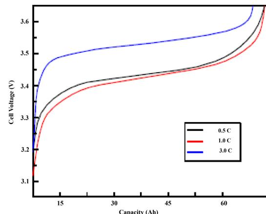
Figure 5: These curves show cell voltage for different charge rates, 0.5 C, 1 C, and 3 C. Nominal cell voltage is 3.2 V. Data provided by Elite Power Solutions.
