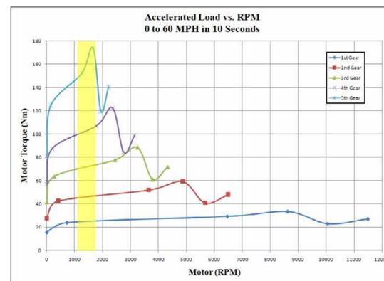
Figure 3: Predicted torque needed to accelerate a 1900 kg EV from 0 to 60 MPH in 10 seconds using a GM 2.2 L, 5-speed transmission. Speeds between 1200 to 1778 RPM are highlighted in yellow where the traction motor produces the most torque. This traction motor is rated for a maximum of 5000 RPM.
