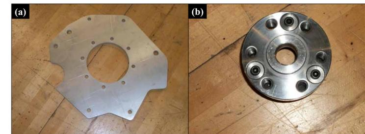
Figure 9: Picture (a) shows the mounting plate used to secure the electric motor to the 5-speed transmission. The mounting plate was fabricated using a water jet cutter by the Rheem corporation. Picture (b) shows the custom flywheel hub designed to secure the flywheel to the electric motor shaft.
