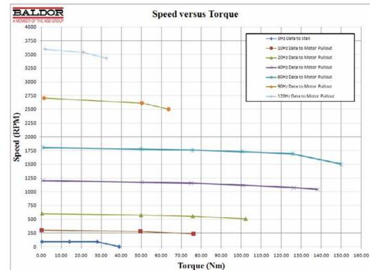
Figure 1: Torque produced by customized traction motor used in second generation Electric Vehicle (EV). This motor produces maximum torque between 1200 to 1780 RPM.
