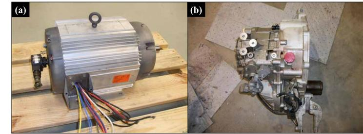
Figure 7: Photographs showing customized motor (a) designed for second generation BEV and 5-speed manual transmission (b) used in the new design.
