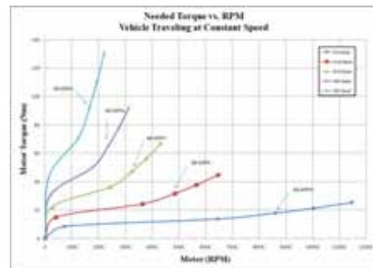
Figure 4: This figure shows the predicted torques needed to maintain EV speed. The EV is 1900 kg and uses the transmission described in Figure 3. Rolling and air resistance was taken into account with these values.
