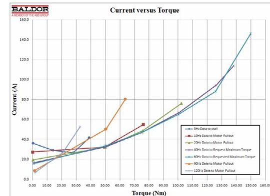
Figure 2: Motor current needed to produce demanded torque in this electric vehicle application. Current demands fall within capabilities of Li batteries and motor controller.
