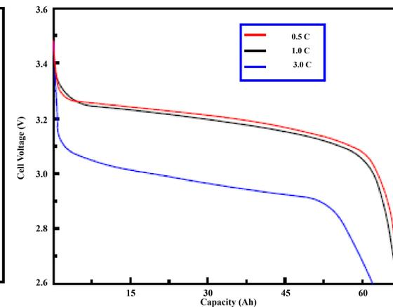
Figure 6: These curves show cell voltage for different discharge rates, 0.5 C, 1 C, and 3 C. Nominal cell voltage is 3.2 V. Data provided by Elite Power Solutions.
