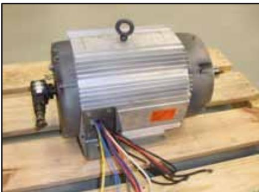
Figure 5: Photographs showing customized motor designed for second generation BEV and 5-speed manual transmission.
