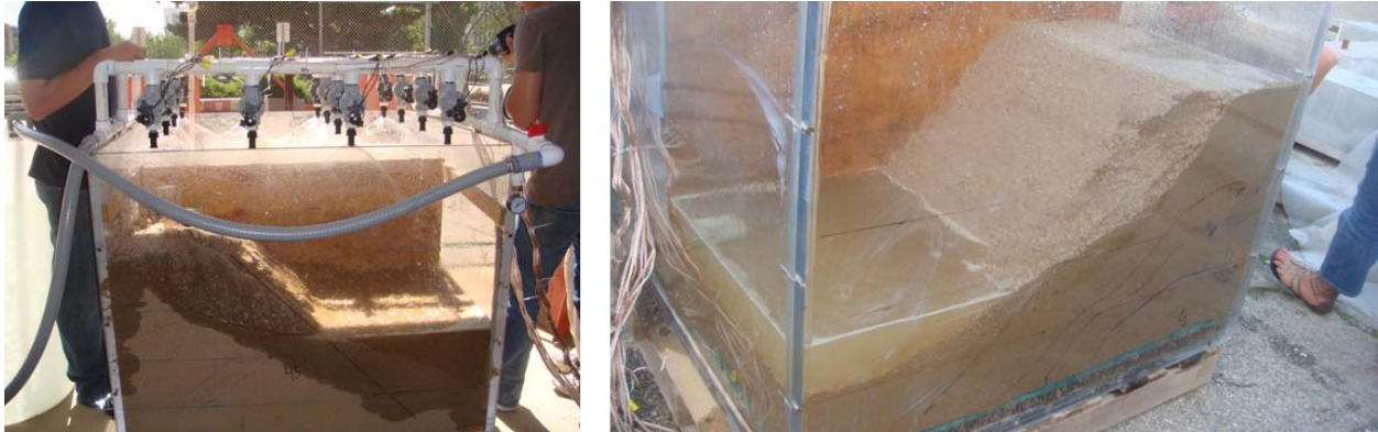
Figure 4: Left: Seepage of rainwater in the soil strata to cause softening in soil; Right: Ponding water and soil erosion after excessive rainfall.
