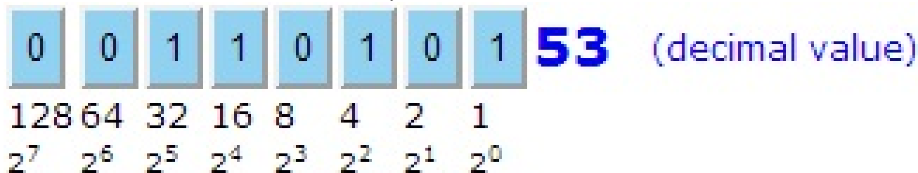
Figure 1: Binary-to-decimal converter activity allows students to toggle each bit of a binary number with a click and instantly show the decimal value.
