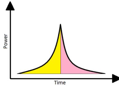
Figure 15. Power Consumption behavior for Gate-to-Drain Breakdown
