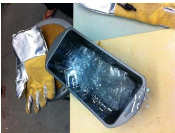
Figure 5: Cut plastic bottles prepared for the first recycling pilot experiment.
