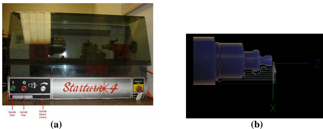
Figure 1. Tabletop CNC lathe: (a) Retrofitted and functional; (b) Artifact made 1
