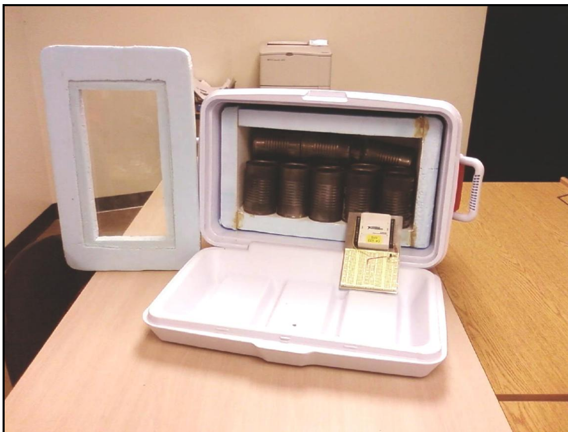
Figure 2. ENGR 3045 Engineering Design Lab I, “Junior Design I,” Fall 2008, Passive Solar Home (1/24-Scale), Thermal Mass (Water), Window, Data Acquisition System
