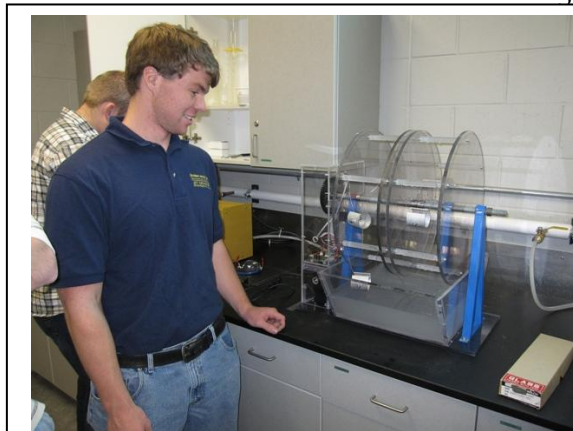
Figure 2. Device for alternating soaking and drying of corrosion test specimens.
