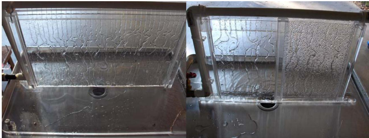
Figure 8. The wet wall module, single-wall on left, double-wall on right.
