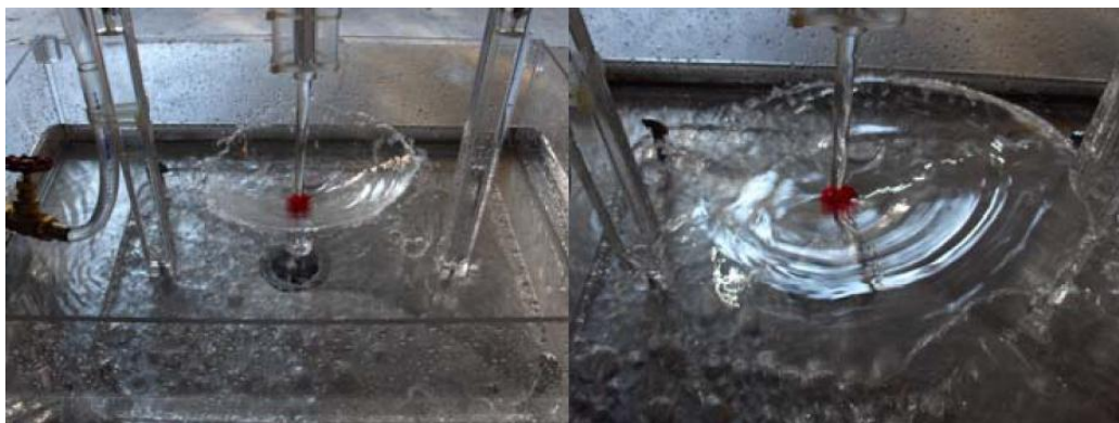
Figure 7. Water sheets produced by a concave impactor; effect of higher flow rate shown on the right.
