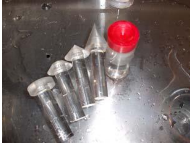
Figure 4. Impactors shown from left are: a flat disk, cones of different angles, and the red concave impactor in the holder. The impactor diameter is 1 in.
