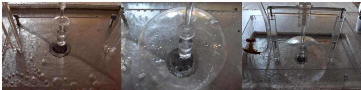
Figure 5. Water bells created by 1in flat disk impactor. From left to right, low, medium and high flow rates. Scales not the same in the three photographs.
