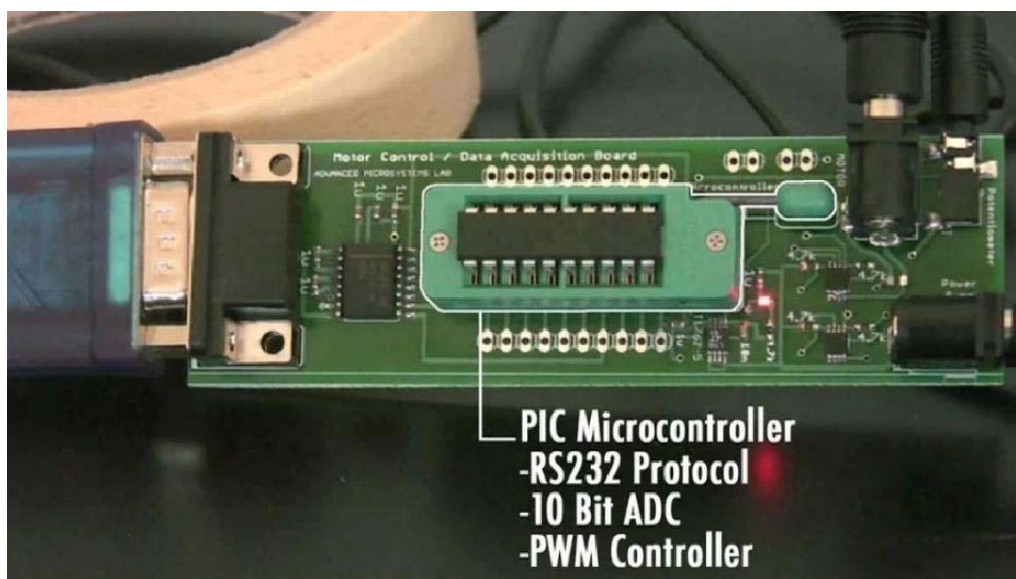
Fig. 2: Circuit board controlling the motor and reading the potentiometer voltage
