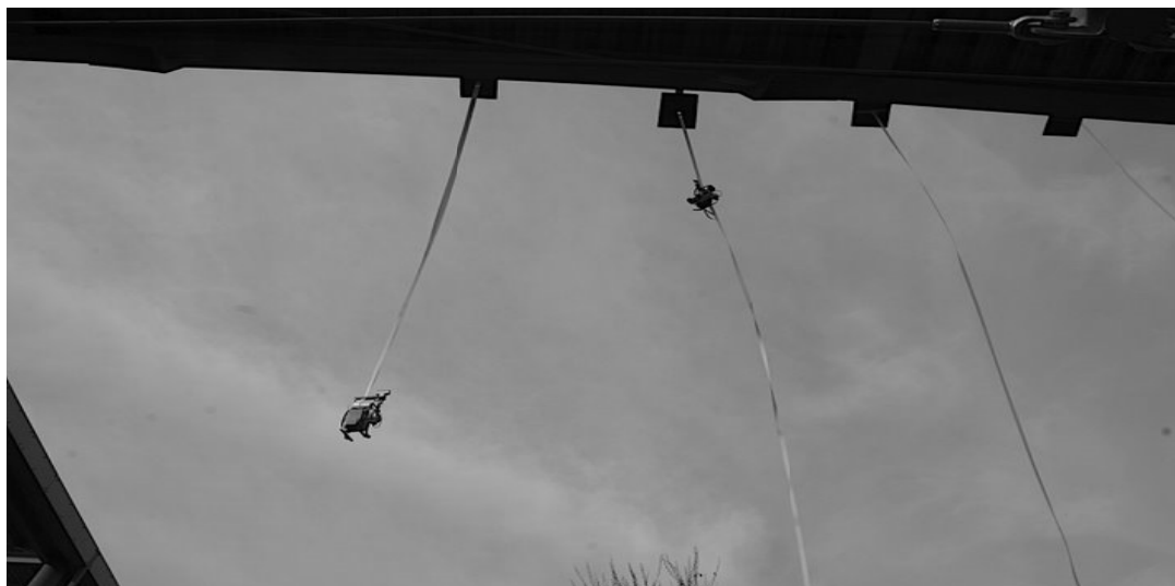
Figure 3: Ribbon set up with two robots attempting to complete their goals. Note one robot is winding the ribbon while the other is rolling along the ribbon [3] .
