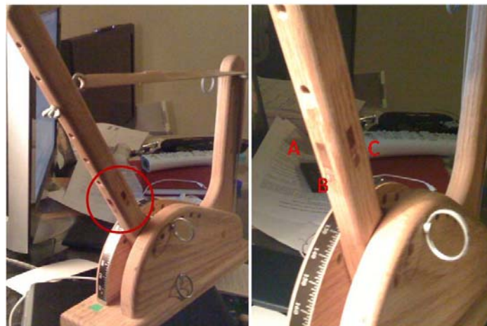
Figure 5. Initial Strain Gage Setup. Gages C and A (not shown) measure axial stress in a half Wheatstone bridge. Gage B is a redundant gage that can potentially be used to capture bending.
