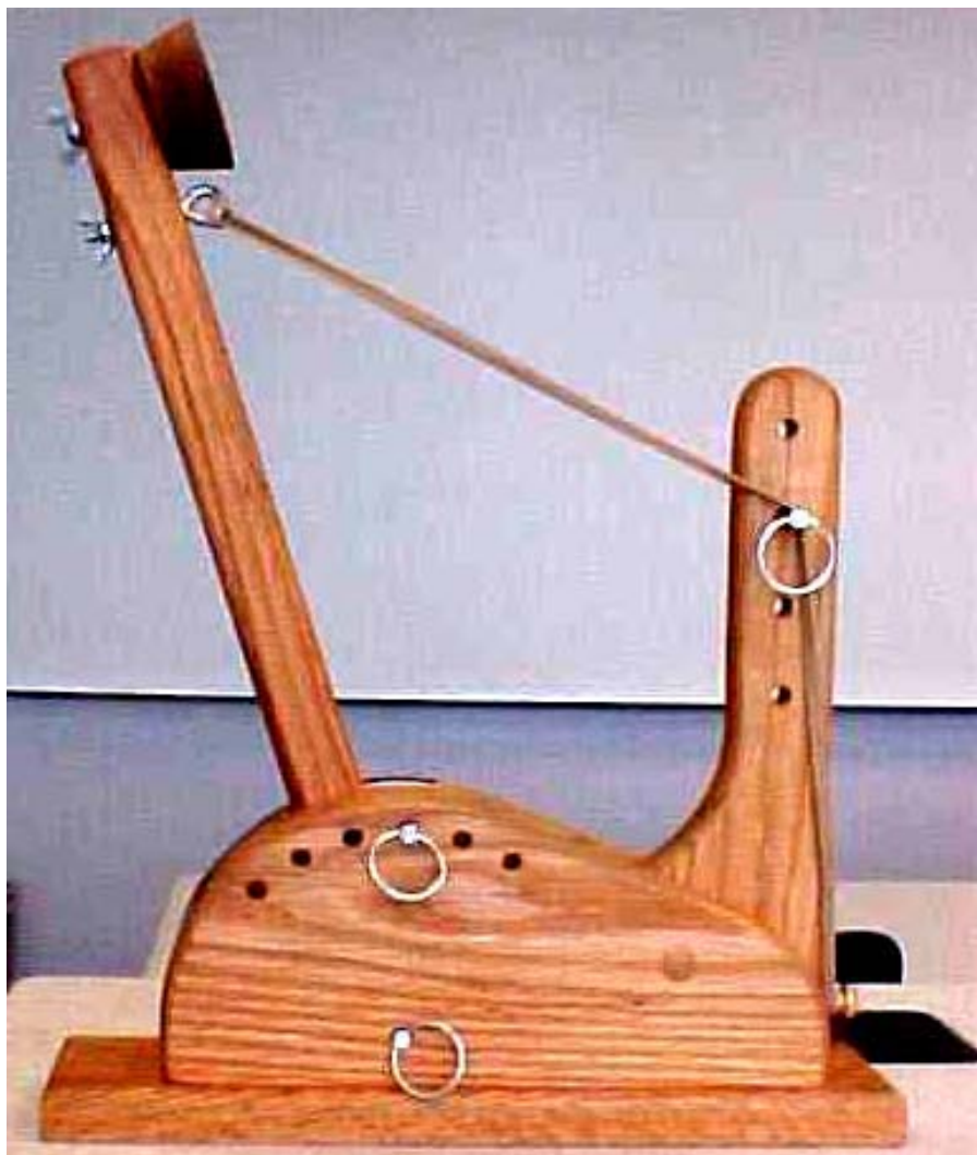
Figure 1: The Statapult, designed as a Six Sigma quality management training device available for purchase online.
