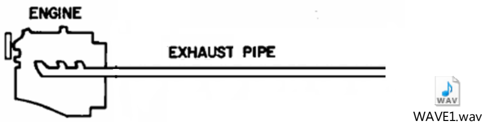
Fig. 13: Typical exhaust system without muffler element
