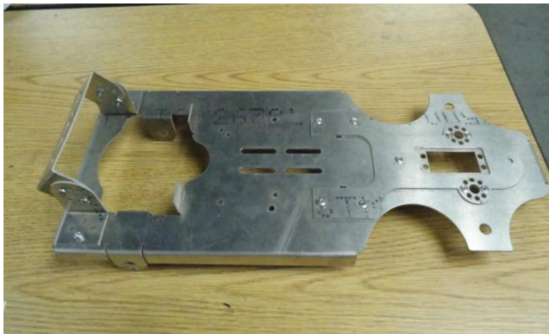
Figure 2: An actual chassis made of sheet metal
