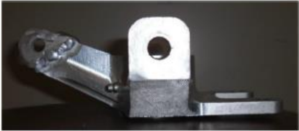
Figure 6: A photo of the broken front knuckle.
