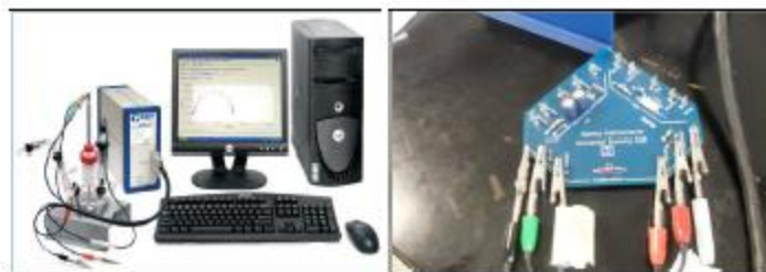
Figure 1: Gamry Reference 600 EIS System Figure 2: Dummy cell with 2 k \Omega resistor. (Electrochemical impedance spectroscopy) [14]
