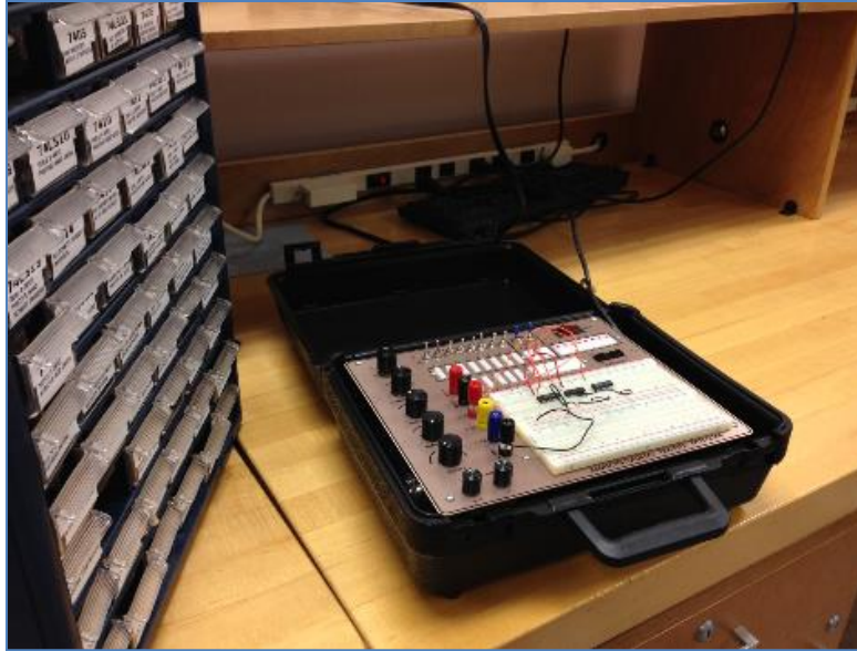
Figure 1. Digital Logic Circuit lab with TTL chips on traditional breadboard
