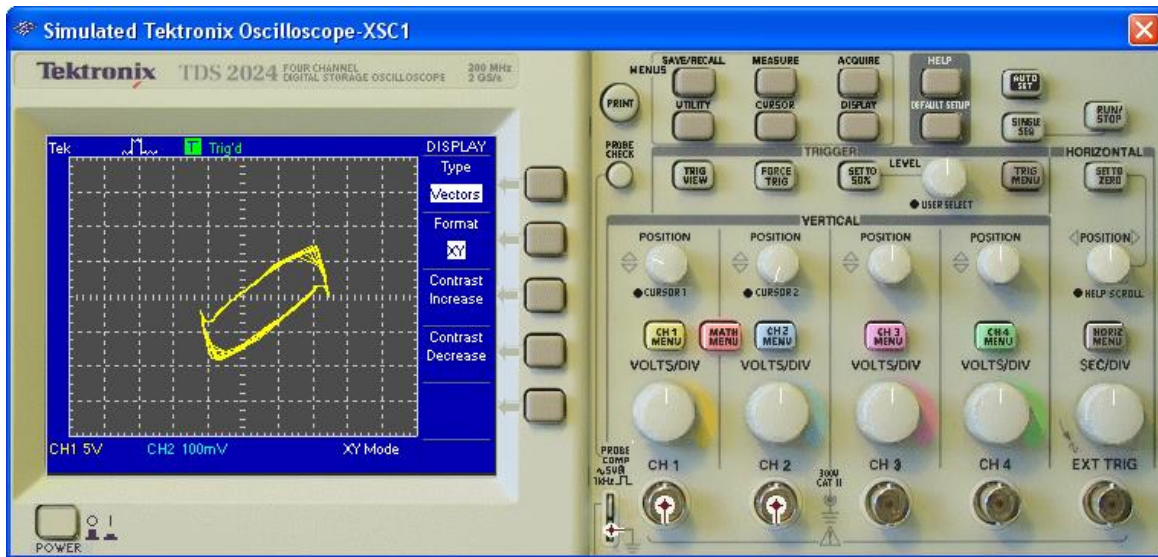
Fig. 4(b). Phase portrait of the probed signals V_{c1} versus V_r
