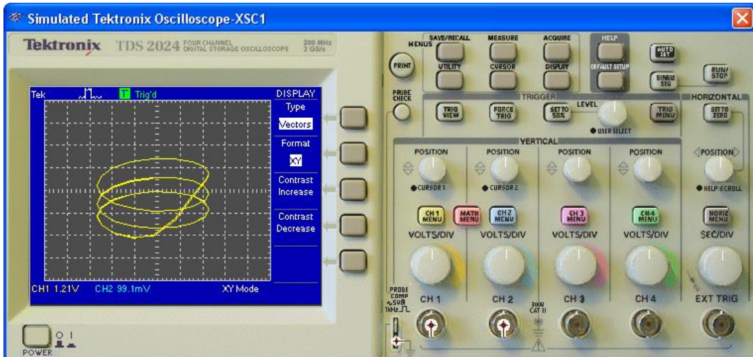
Fig. 3(c). Phase portrait of V_{in} versus V_R
