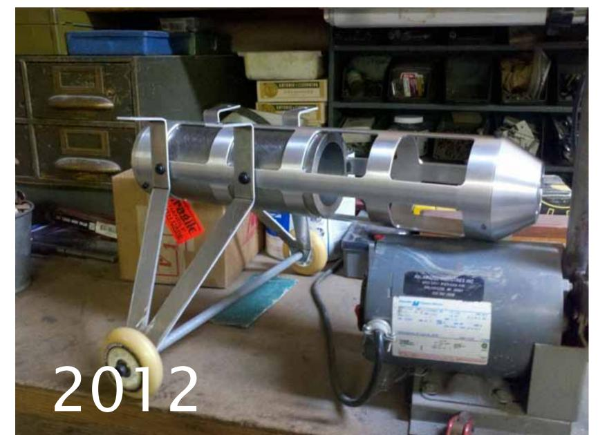
can lift. Therefore, the more weight that a team can remove from its plane, the more payload they can lift. For the 2012 season, Kansas State University's Aero Design Team focused on reducing weight from a basic design that had proven successful in the past. The landing gear design focused on reducing the number of components to reduce weight. By combining the wing mount and landing gear, the number of parts was reduced from thirteen to three. This reduced weight by 45%.
