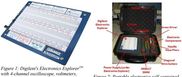
with 4-channel oscilloscope, voltmeters, voltage sources, waveform generator and logic analyzer.
