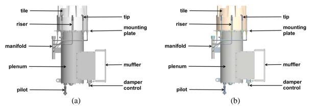
Figure 6. 2D drawings of a process burner: (a) black-and-white and (b) color.
