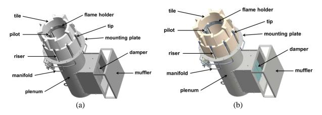
Figure 7. 3D drawings of a process burner: (a) black-and-white and (b) color.
