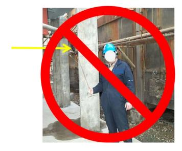
Figure 10. Photograph of an operator holding a rag on a stick, which is improperly used to light a process burner.
