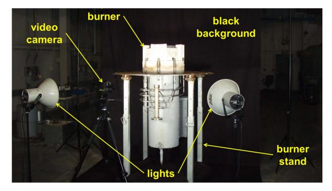
Figure 4. Setup for taking a video of the burner.
