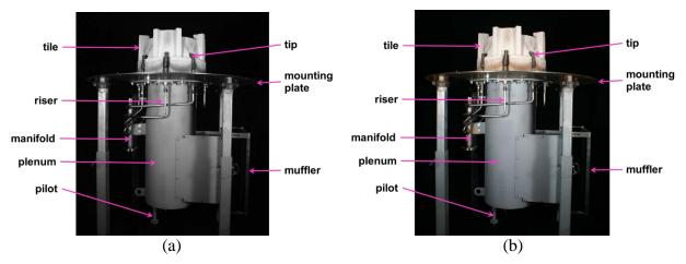
Figure 5. Photographs of a process burner: (a) black-and-white and (b) color.
