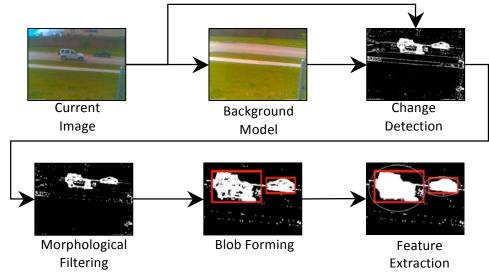
Figure 2. Block diagram of video processing pipeline.
