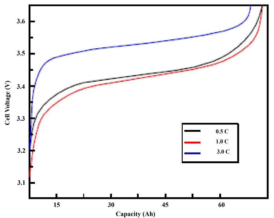
**Figure 5: These curves show cell voltage for different charge** rates, 0.5 C, 1 C, and 3 C. Nominal cell voltage is 3.2 V. **Data provided by Elite Power Solutions.**
