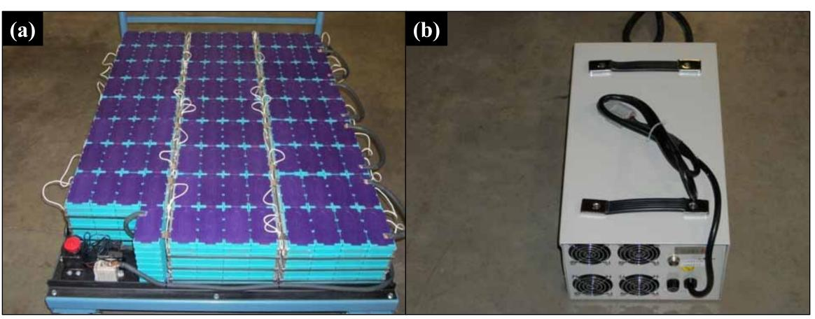
Figure 8: Photograph (a) shows the LiFeMnPO4 battery pack used in the second generation EV and (b) custom 105 cell battery charger on the right. The batteries can be recharged using a standard 120/240 V electrical outlet. This battery bank will eventually be placed in the trunk of the second generation EV.
