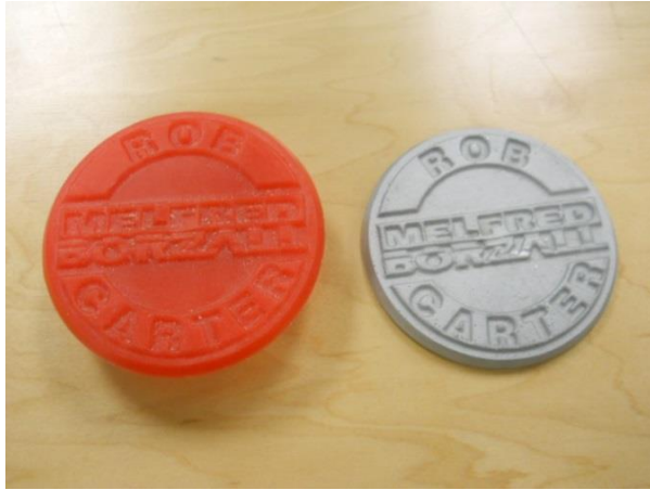
Figure 21) Machined Pattern and Casting
