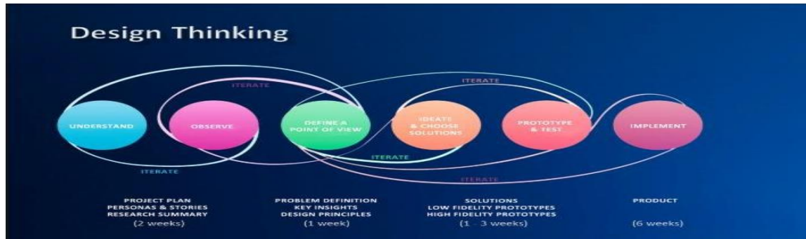
Figure 9: Design thinking is an experimental and iterative process 10
