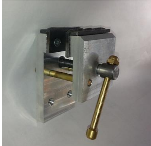
Figure 3. Final product: Multiple materials and COTS components all shown.
