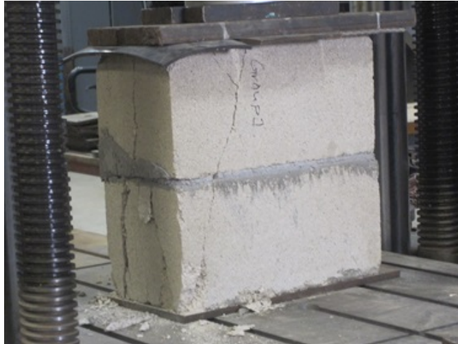
Figure 8: Compressive testing of masonry prism
